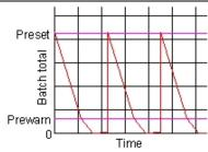
In down-counting batch control, the Laureate counts down from the preset maximum to zero. A prewarn level is available to slow down filling or emptying near zero. Again, a time delay can be programmed from the end of each batch to the start of the next batch.
