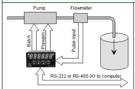
In this drum filling application, the Laureate pulseinput batch controller utilizes uses its two relays to control a pump. The Prewarn relay slows down the pump near the preset to avoid overshoot. The Batch relay stops the pump at the preset.
