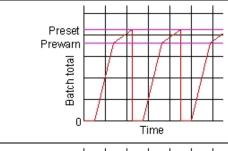
In up-counting batch control, the Laureate counts up from zero to a preset maximum. A prewarn level is available to slow down filling near the preset to avoid overshoot. A time delay can be programmed from the end of each batch to the start of the next batch.
