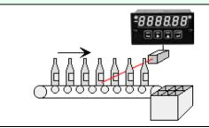
The Laureate batch controller is ideal for discrete manufacturing as well as repetitive fill operations. In this example, the Laureate counts bottles which it then groups into sixpacks. Its Grand Total capability can be used to track bottles or sixpacks.
