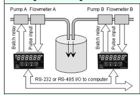
Multiple Laureate batch controllers can be used in combination to control the mixing of materials in the proper ratio. Each feed line is equipped with its own pump, flowmeter, and Laureate.
