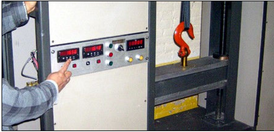
Seat belt tensile strength testing using Laureate digital panel meters. The three meters display Force, Displacement and Speed.
