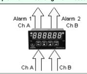
A single Laureate dual-channel counter will handle two repetitive fill operations by counting from zero up to a preset, or down from a preset to zero. A dual setpoint relay board is required.
