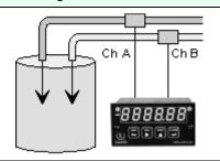
A+B, A-B and A/B arithmetic functions are available with the Extended counter. A+B sums both totals, while A-B subtracts the outflow total from inflow total. The A/B ratio applied to total helps assure the proper mixing of components.
