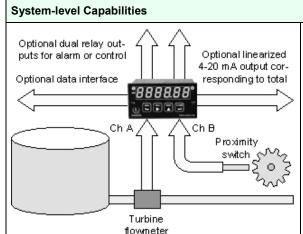
The Laureate dual channel totalizer can independently scale, display and alarm two totals, and the totals plus alarm data can be transmitted via RS-232 or RS-485. The displayed totals can also be transmitted as an isolated 4-20 mA or 0-10V analog output. The Extended version can further display and transmit arithmetic combinations of the two totals.
