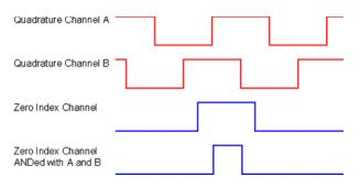
The Laureate quadrature transmitter accepts A & B quadrature encoder signals to provide an analog output that tracks position, length, angle, or rate. The A & B quadrature signals are 90° out of phase, and their phase relationship determines whether up counts (+) or down counts (-) are produced.
