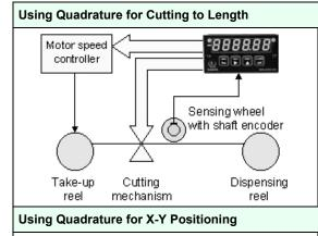
Controlling the repetitive cutting of material to length is an excellent application of a Laureate quadrature transmitter or Laureate quadrature meter. The quadrature encoder shares the shaft of a sensing wheel, whose rotation corresponds to lineal displacement of material. The transmitter compares the displacement reading against setpoint information, and then uses its dual relays to first slow down and then cut the material.
