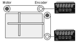
Accurate X-Y position or rate can be obtained from two shaft encoders, which convert linear position to quadrature signals as a shaft turns. In addition to serving as a transmitter, each Laureate transmitter or meter can use its optional dual relay setpoint capability for closed loop control.
