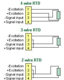
In 4-wire hookup, different pairs of leads are used to apply the excitation current and sense the voltage drop across the RTD, so that the IR drop across the excitation leads is not a factor.
