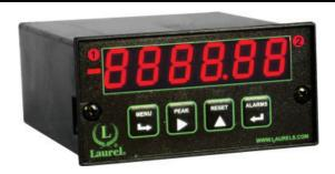
Laureate™ six-digit remote displays accept serial data from a computer, PLC or other instrument to display a numeric reading from -999,999 to +999,999. The units match the appearance of Laureate digital panel meters and counters. The display consists of six 14.2 mm (.56") high LED digits, available in red or green. The 1/8 DIN front panel is environmentally sealed to NEMA-4X when panel mounted.
