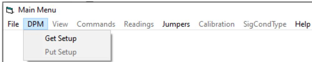
With your instrument communicating, the second from the left item in the top ribbon will be DPM or Counter, depending on whether IS software has detected an analog input instrument or pulse input instrument. Click on that heading.
