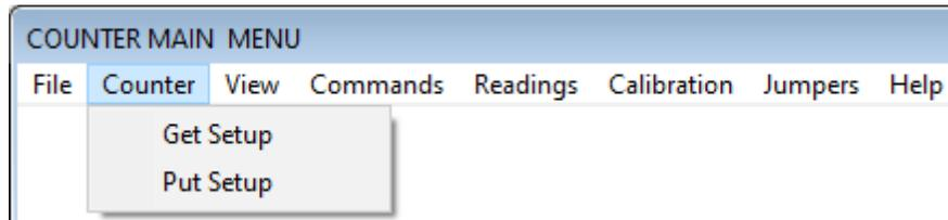
**DPM or Counter** will be the heading in the top menu bar, depending on whether the instrument has been detected as an analog input DPM or a pulse input counter.
