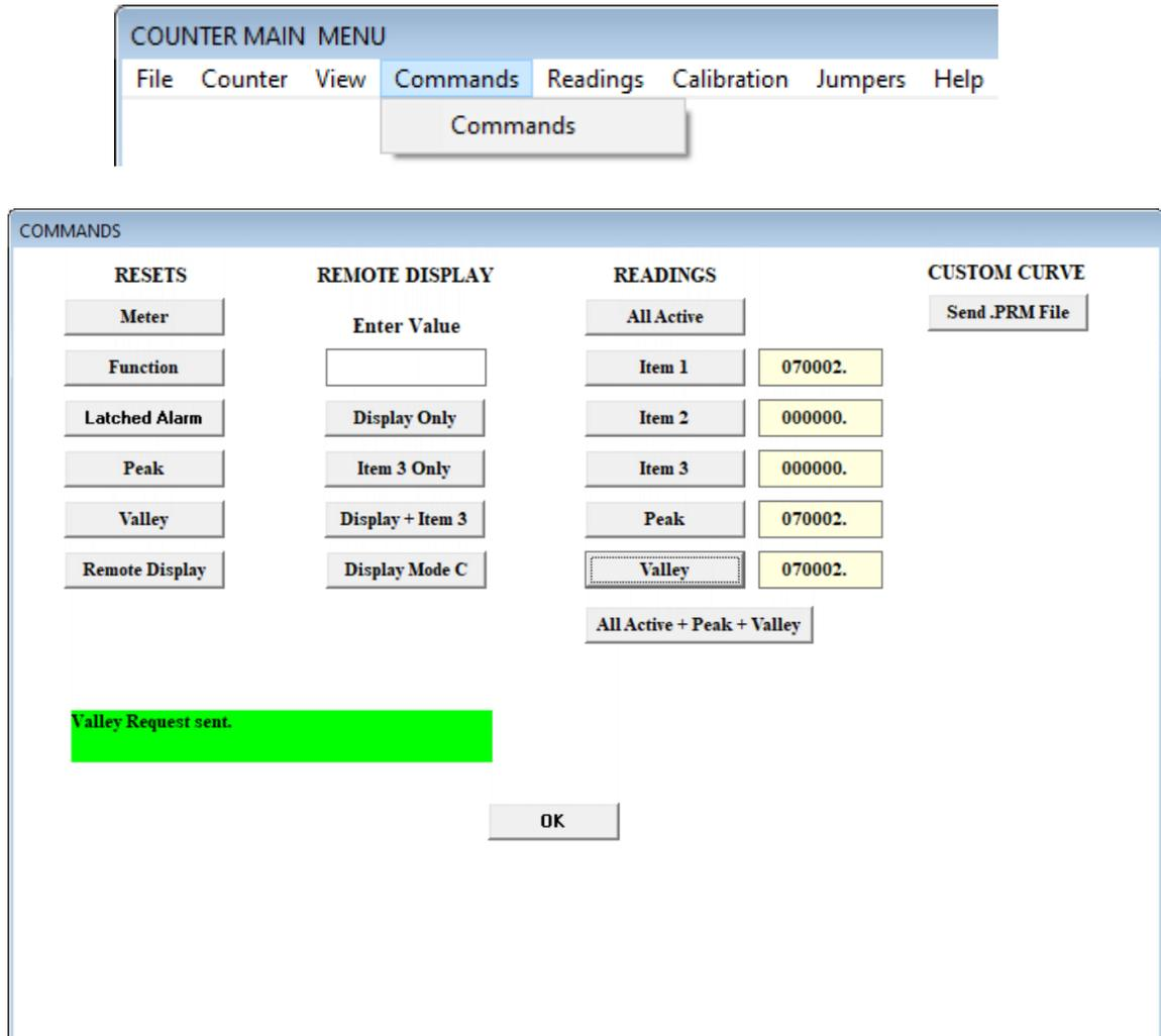
**The Commands Selection**, illustrated here for the Laureate counter, allows the PC running IS software to perform specific tasks at the push of a mouse button. These tasks could otherwise be performed from a meter's front panel, from external control inputs, or by sending commands with the Custom ASCII or Modbus protocol.
