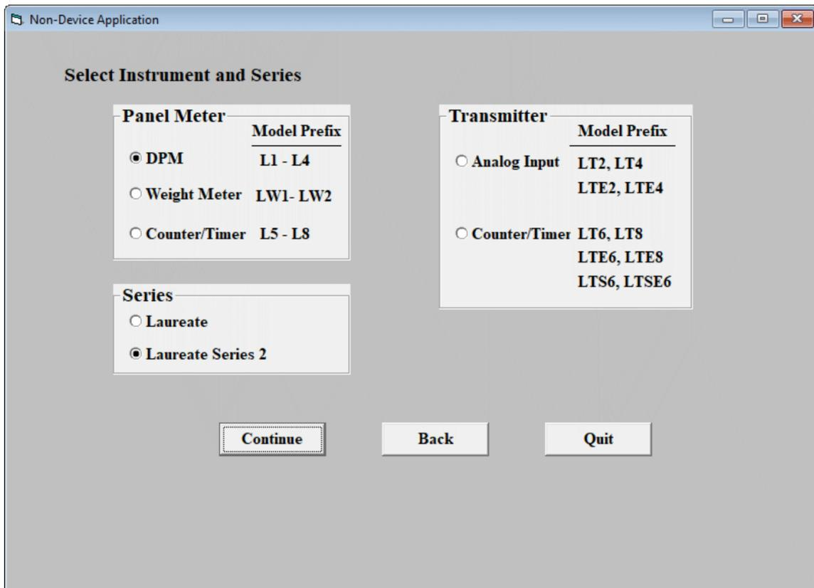
If your instrument is a panel meter, select DPM, Weight Meter or Counter/Timer, and select “Laureate Series 2.” If your instrument is a transmitter, select “Analog Input” or Counter/timer. Click on Continue, then on “Default Setup” in the Counter Main Menu.
