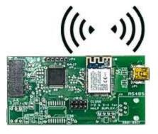
LWIFIX has the same capabilities as LWIFI but comes with an external 5 dBi antenna and a 30" antenna cable instead of a printed internal antenna. Use of an external antenna allows meter installation inside a metal cabinet and increases range up to 30 m (100 ft).
