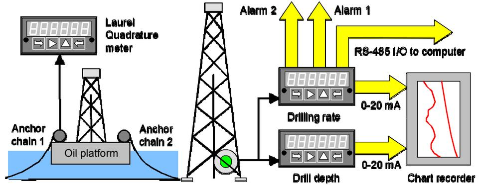
Once drilling has begun, there is the additional challenge of accurately measuring the length of drilling shaft that has been sunk into the seabed and reading out the rate of drilling in feet per hour as the drill makes it way through different layers of sedimentary rock. High vibration would
