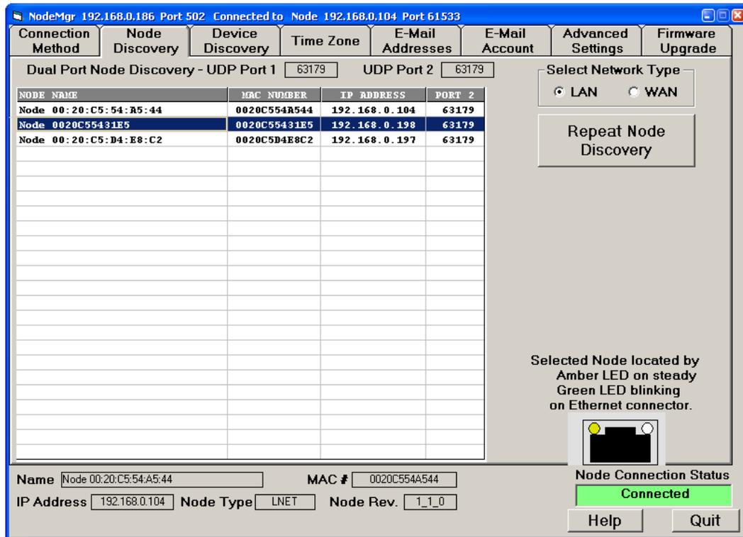
Nodes on a local LAN are automatically discovered under the Node Discovery tab when “LAN” is selected under “Select Network Type”. Nodes can be rediscovered at any time by pressing the “Repeat Node Discovery” button. Your Windows firewall settings must allow Node Manager Software to run, or Nodes will not be discovered. Check with your IT department if you suspect a firewall issue.
