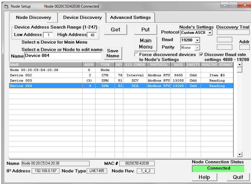
To discover remote devices on an RS485 bus interconnected by Laurel's GBL03 data cables:
