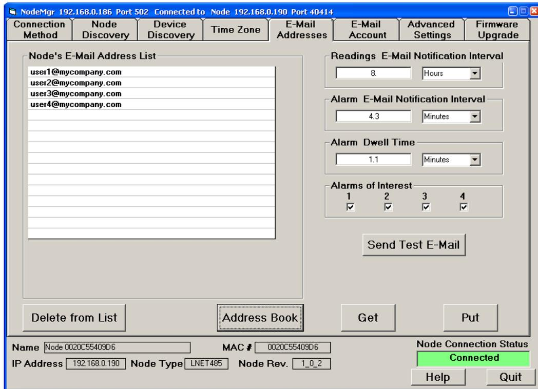
Readings and alarm notifications can be emailed by the Node to a list of email addresses stored in the Node.
