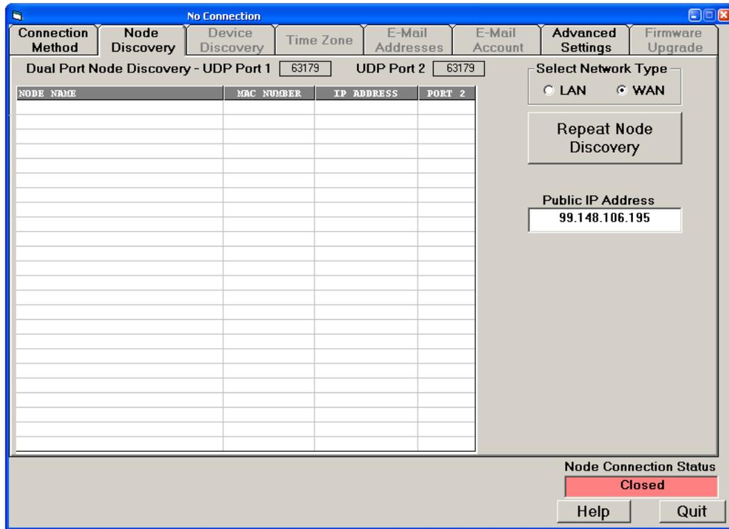
Nodes on a remote LAN are automatically discovered via the Internet by selecting “WAN” under “Select Network Type”, entering the Public IP Address of the router to which the Nodes are connected, and pressing on “Repeat Node Discovery”.
