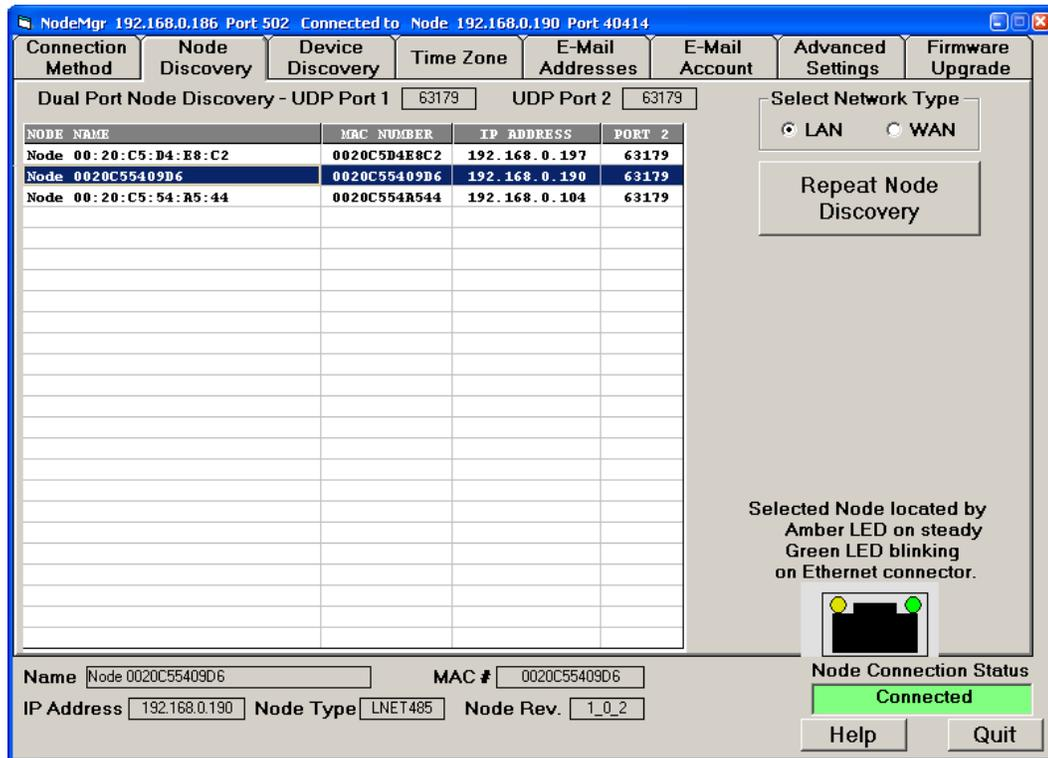
If the selected Node is the LNET485 Ethernet-to-serial device server option board of a meter, up to 31 RS485 physical devices may be discovered, including the host meter of the LNET485 option board. Since Modbus allows addresses of 1-247, there can be unused addresses.
