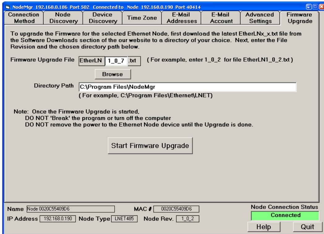
Node firmware upgrades are available from the factory at no charge and should be installed into each Node when available. Upgrading the firmware will not affect data stored in the Node.
