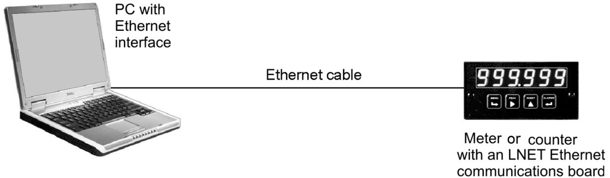
**Example 1.** The host PC has a direct Ethernet cable connection to a Laureate meter or counter with an LNET Ethernet board or to an LTE series transmitter. This is an easy way to program the Laureate using Instrument Setup software or to datalog readings from the Laureate to a PC using XLog2 Datalogging software.
