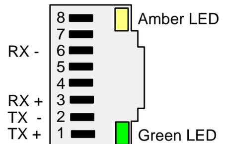
Ethernet cables (CAT5 or better) can be straight-through or crossover. Our Ethernet Nodes automatically adapt for either.
