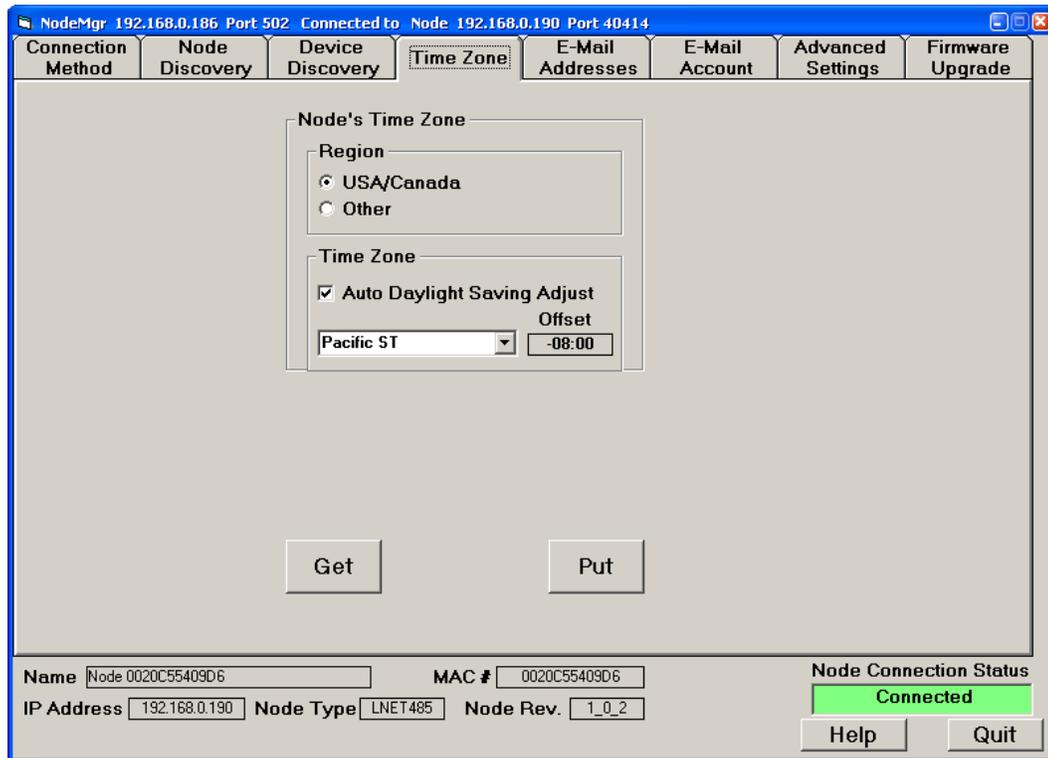
A time stamp is included in email messages and in streaming data sent by the Node. If the Node has a path to the Internet (also required for email), the Node will automatically obtain accurate UTC/GMT time (Coordinated Universal Time or Greenwich Mean Time) from an online time server. The Node's time zone or the offset from UTC/GMT time must be also supplied using this screen.
