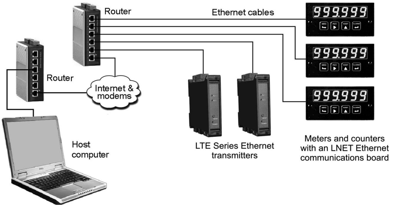
**Example 3.** For connection via the Internet, the PC can be plugged into a local LAN, and remote instruments can be plugged into a remote LAN. When the IP address of the remote router is supplied, Laureate Ethernet Nodes and any Devices attached to them via an RS485 bus are automatically discovered by our Node Manager software, Instrument Setup Software, or XLog2 Datalogging software.
