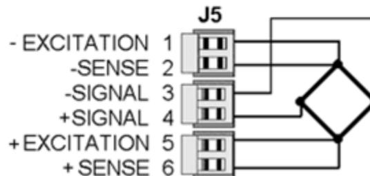
Excitation voltage can be jumpered for 5, 10 or 24 Vdc (Section 17).
